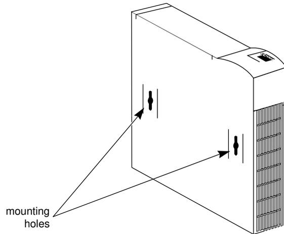
These slots fit over the heads of wall-mounting screws to secure the modem to the wall. A mounting template for marking the location of the mounting screws is included in the foldout *Installation Guide* that accompanies this manual.
