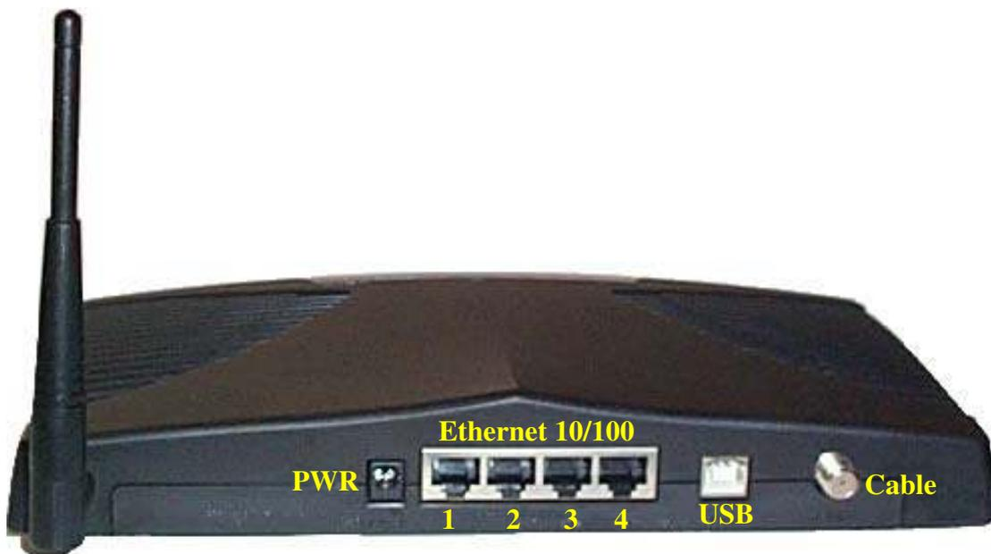
1. **PWR:** This is where you plug the included power adapter. Remember to use only the power adapter that came with the wireless cable modem.
