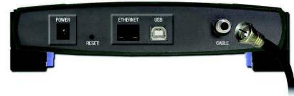
Figure 3-3: Connect the Coaxial Cable
