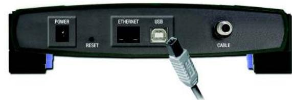
Figure 3-4: Connect the USB Cable
