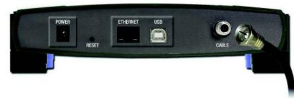
Figure 3-1: Connect the Coaxial Cable
